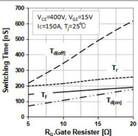
Typical switching times as a function of gate resistor
