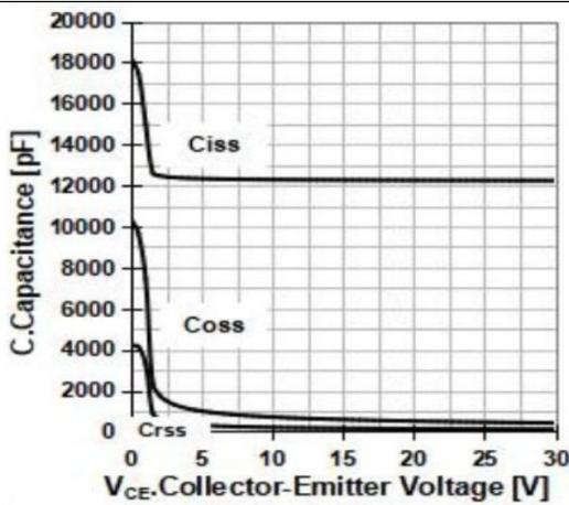
Typical capacitance as a function of collector-emitter voltage
