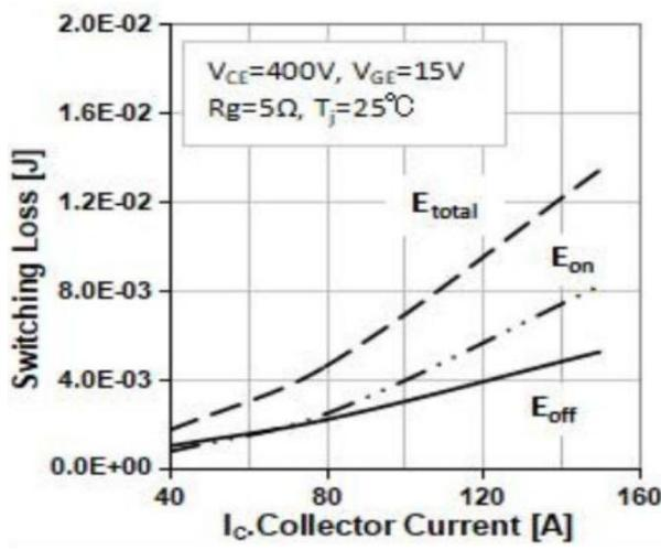
Typical switching energy losses as a function of Collector Current
