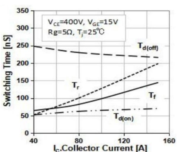
Typical switching times as a function of Collector Current
