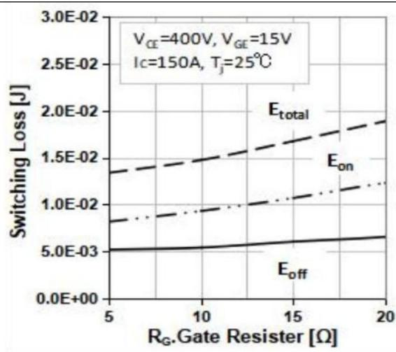
Typical switching energy losses as a function of gate resistor
